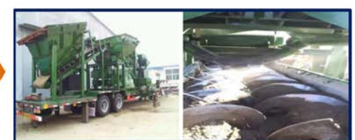
(MIXING SOIL WITH HARDENER & CEMENT)
